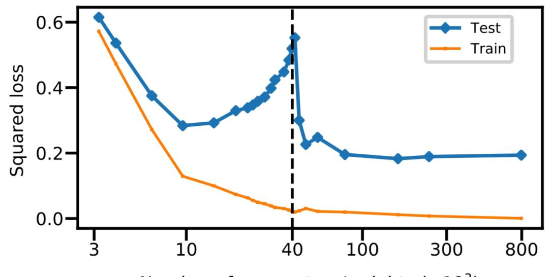
Figure 4: Double descent risk curve for fully connected neural network on MNIST. [Belkin et al, 2019]
